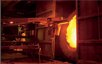
LaCam® - C I (fixed installation) at a converter
