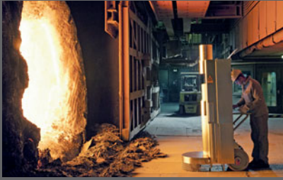
LaCam® - M mobile version for converter and ladles for extremely high ambient temperature
