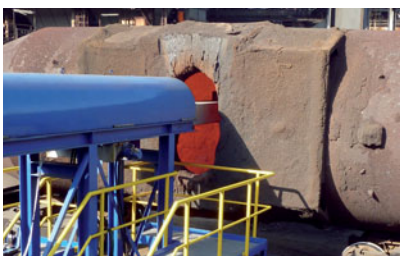
LaCam® - Torpedo (fixed installation) at torpedo ladles
