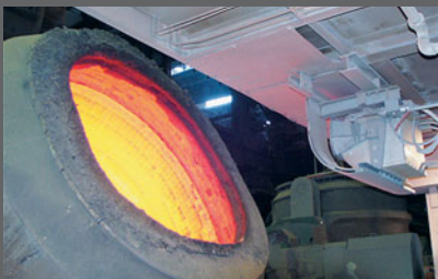
LaCam® - L I (fixed installation) at a ladle stand
