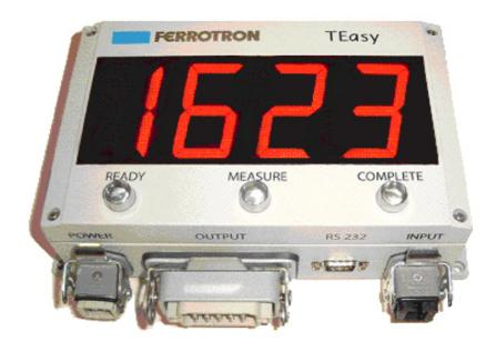
Microprocessor controlled temperature measuring device, performed in a dust- and splash-proof sheet enclosure for wall mounting, sturdy design, with large 55 mm character height LED-display (4 decades) to indicate the temperature values available for thermocouples type: Pt 10 (S) or Pt 13 (R) and Pt30Rh (B) factory presetted.
