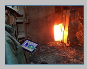
Users use remote control to operate the **LaShot 4**, and the standard operation is to touch the tablet computer with 12.3 inches, which is the most suitable and simple way to operate the device. Remote operation through an 11 Mbit wireless network, two USB interface in the connection board, a 1000 Mbit Ethernet connection. Ethernet connection is mainly used to connect with local area network in steel plant, which can be used to share equipment measurement data.
