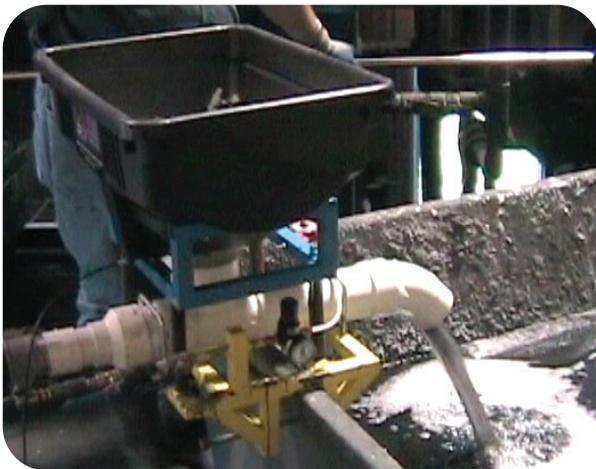
Latex flowing through LiquiSorb feeder mounted to dump cart
