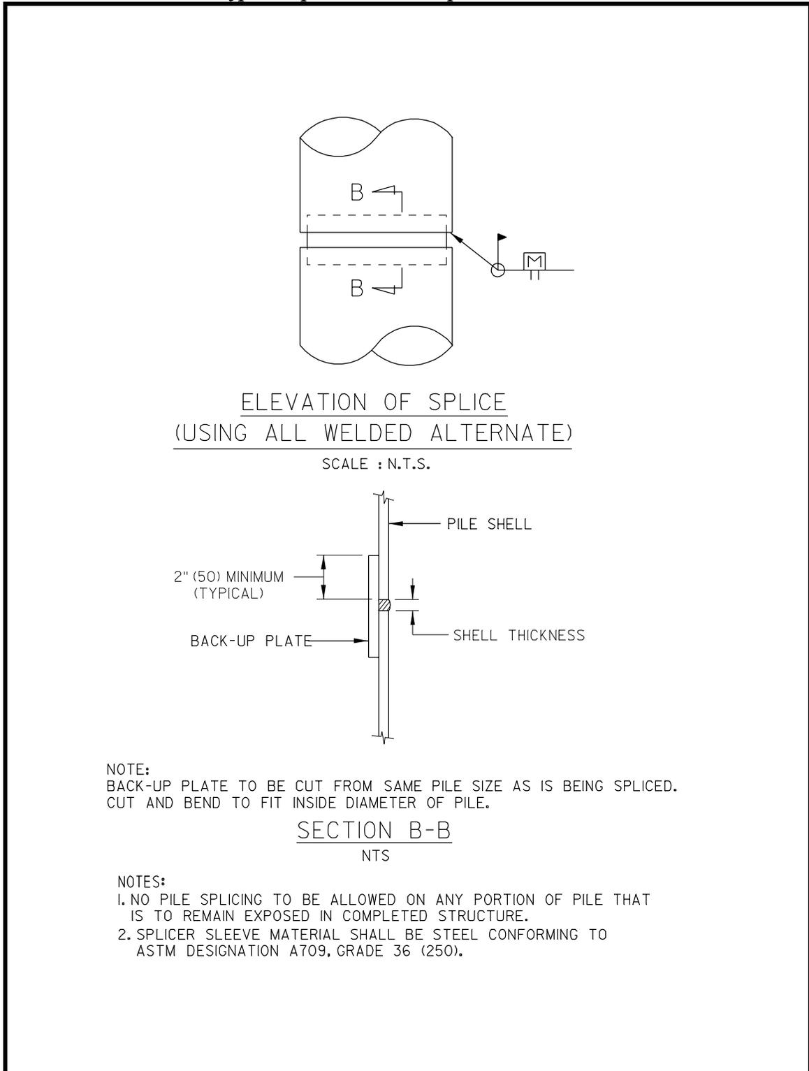
Steel pipe piles can be used as friction, point bearing or rock-socketed piles. They are commonly used where variable pile lengths are required because splicing is relatively easy. As noted in Section 6.2.2.1, piles should not be used where the depth to bedrock is less than 10 ft. [3 m].
