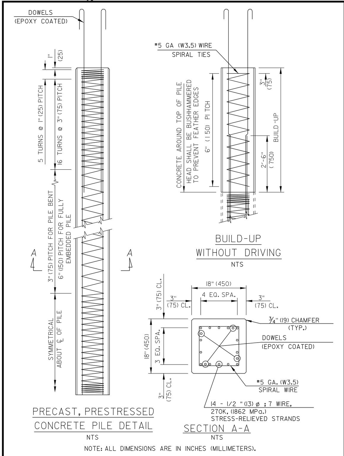
The primary advantage of prestressed concrete piles over conventional reinforced concrete piles is durability. Because the concrete is under continuous compression, hairline cracks are kept tightly closed and thus prestressed piles are usually more durable than conventionally reinforced piles. Another advantage of prestressing (compression) is that the tensile stresses which can develop in the concrete under certain driving conditions are less critical.
