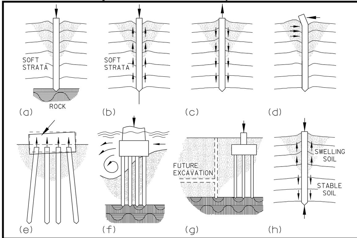
Negative skin friction occurs where the soil surrounding the pile exhibits a downward movement with respect to the pile shaft. There are various causes of the downward movement of the soil. All the causes increase the load on the pile. This is also known as downdrag and is analyzed as additional axial load.
