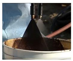
Spray applied LIQUID BOOT® 500 effectively seals the surface of BASEFABRIC T-60 and other irregular surfaces that are considered critical vapor intrusion pathways.
