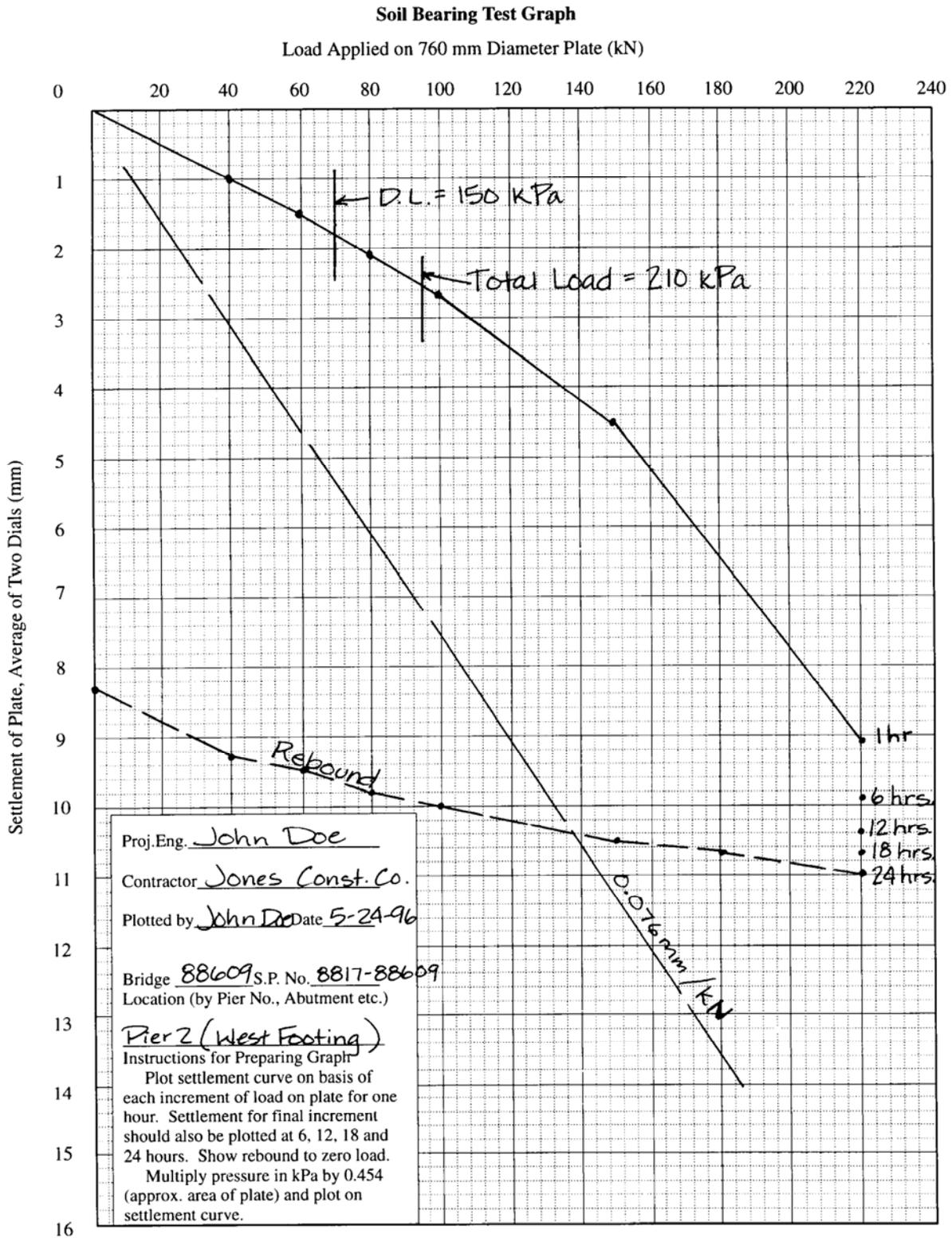
An intelligent determination regarding the adequacy of the supporting soils to support design loads can only be made when complete and accurate information is available from the field. The type of design and the cost of changing to a pile foundation may further influence the final decision. In some cases the dimensions of the footings may be increased to reduce the square-foot loading rather than change to a pile foundation design.
