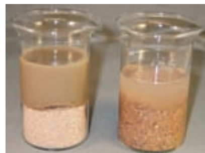
Bentonite and PAC polymer drilling fluid. MINIMAL fluid loss
