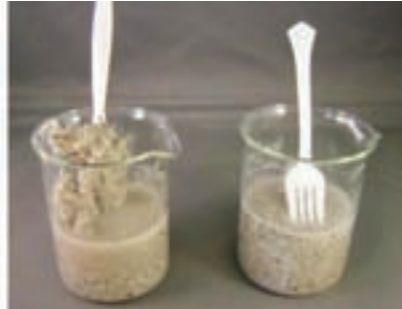
Clay will hydrate, causing sticking and swelling
