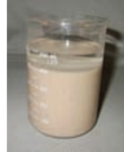
Bentonite settling due to calcium in water
