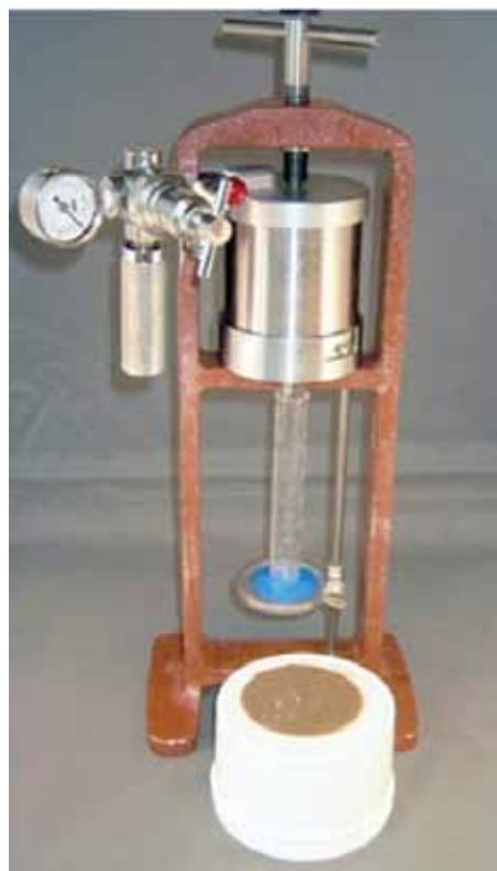
Testing drilling fluid with the filter press.
