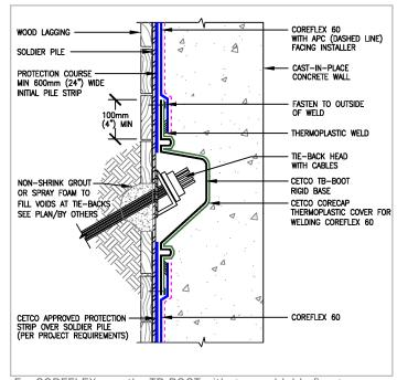
For COREFLEX, use the TB-BOOT with gray weldable flanges installed with COREFLEX field sheet welded to gray flange per CETCO's guidelines
