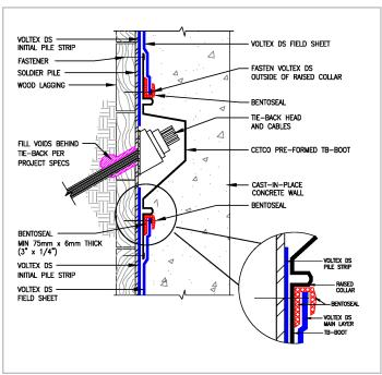
The above detail illustration is applicable for any one of the following CETCO waterproofing membranes per project specifications: VOLTEX, VOLTEX DS, VOLTEX CR, VOLTEX DSCR and ULTRASEAL BT
