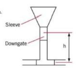
The back pressure in the downgate capacity Q (litres/sec) of the ladle is calculated with Formula 30.
