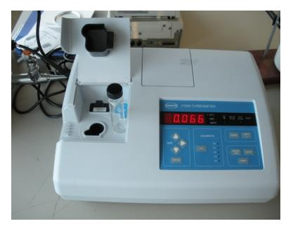
Benchtop model with multiple detector arrangement and accurate between 0-4000 NTU
