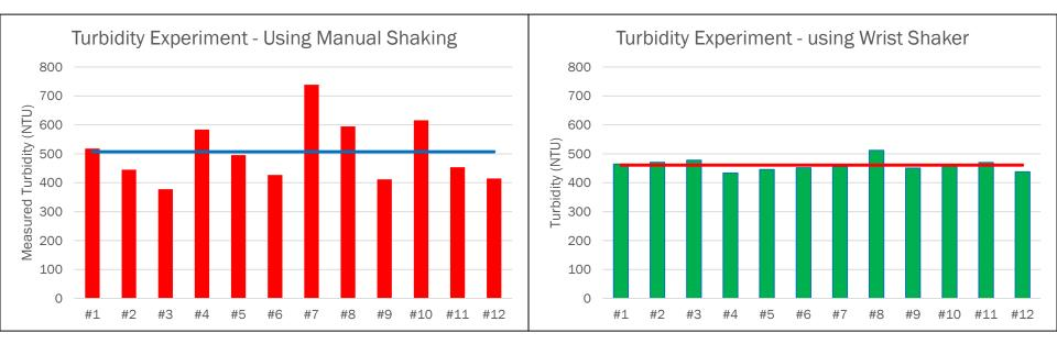
The standard deviation is improved greatly by using a standard , reproducible method of agitation
