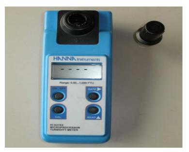
Portable style with single 90° detector- Accurate between 0-100 NTU without need for dilution of sample
