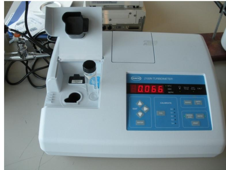
Benchtop model with multiple detector arrangement and accurate between 0-4000 NTU
