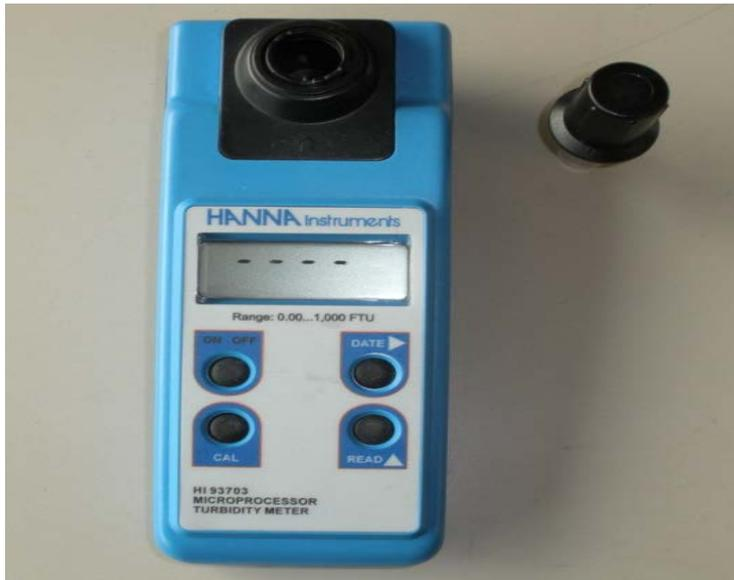
Portable style with single 90° detector- Accurate between 0-100 NTU without need for dilution of sample
