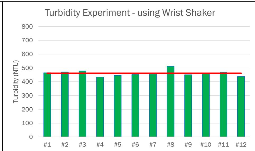
The standard deviation is improved greatly by using a standard , reproducible method of agitation
