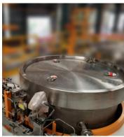
The coalescer vessels are designed to be interchangeable between Hi-Flow® media cartridges and CrudeSorb® MR media cartridges. Both type of canister utilizes the same perforated guide rods connected to the internal header at the bottom of the vessel. This allows the operator adequate flexibility in the event fluid characteristics change (presence of mercury) in the future to ensure environmental discharge limits without production disruptions and without any modifications/disruptions.
