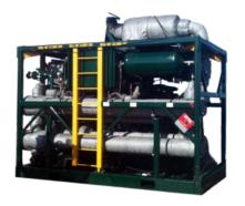
The Tuna™ - Our flameless heat exchanger unit provides a safer solution to fluid temperature control offshore. Unlike other available flameless units which place the recovered well fluid lines inside the open heat source chamber, CETCO's design runs well fluid lines inside a water and glycol bath. This acts as a neutral barrier between recovered well fluids and the unit's heat source to optimize the heating capabilities with an improved design for safety.
