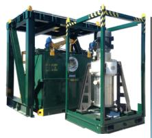
Centrifuges – CETCO centrifuges mechanically separate oil/ water faster than a conventional separator, while using a smaller footprint. This compact unit promotes oil/water separation during flowbacks to return better quality oil for platform sales.
