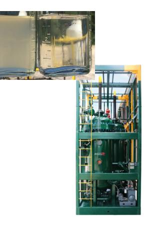
At nominal filtration velocity, ANGLER® CMF has an expected removal efficiency of 80–90% of particles sized 4–5 microns. A 90% or higher efficiency has been achieved with a larger mean particle size range and further optimization.
