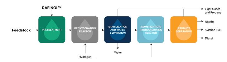
Phosphorous and other metal contaminants have to be removed during pretreatment in order to maximize downstream processes and prolong catalyst life. RAFINOL™ adsorbents offer consistent pretreatment performance across various feedstocks.
