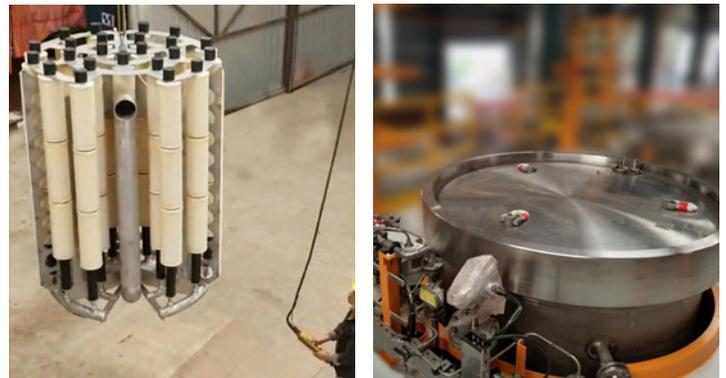
The coalescer vessels are designed to be interchangeable between Hi-Flow® media cartridges and CrudeSorb® MR media cartridges. Both type of canister utilizes the same perforated guide rods connected to the internal header at the bottom of the vessel. This allows the operator adequate flexibility in the event fluid characteristics change (presence of mercury) in the future to ensure environmental discharge limits without production disruptions and without any modifications/disruptions.
