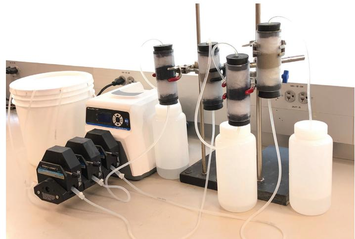
Figure 1 – In-situ stabilization using FLUORO-SORB® with an hydraulic mixing head, and adsorption column study in CETCO's Research and Development Laboratory
